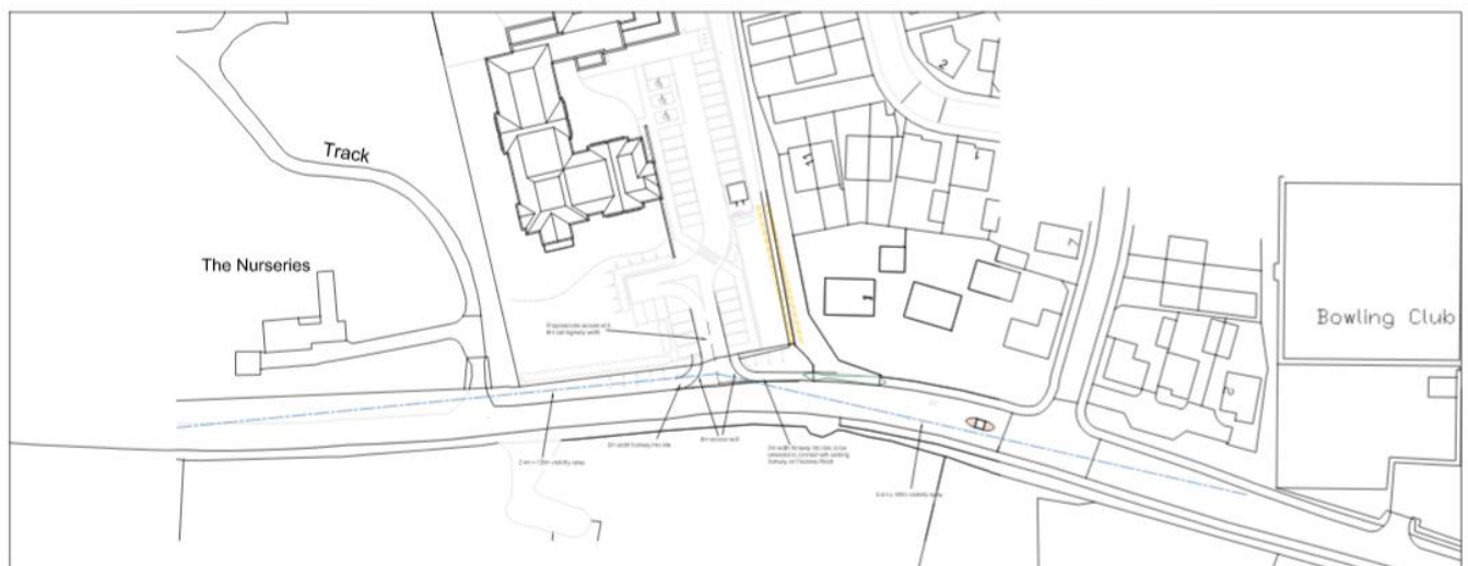
Drawing No. TWCH-BSP-ZZ-XX-DR-S-0001 Rev P02 showing the visibility splay Proposed Site Access Arrangements (1:500)
