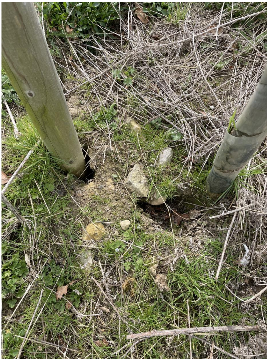
Dried out ground would indicate heavy clay content, large stones also visible.
